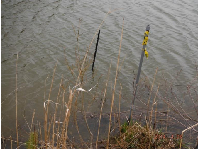
Photograph 11. ↑ Mini-piezometer and staff gauge location.
