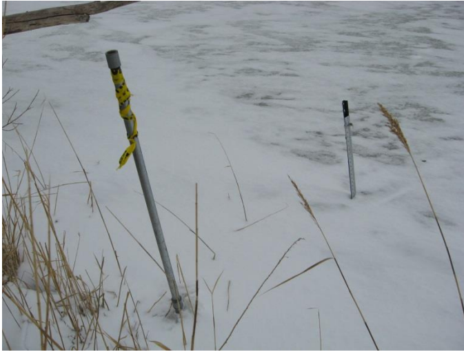
Photograph 11. ↑ Mini-piezometer and staff gauge location.
