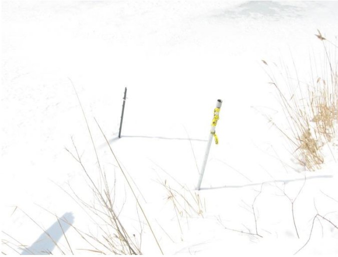
Photograph 11. ↑ Mini-piezometer and staff gauge location, covered in snow.
