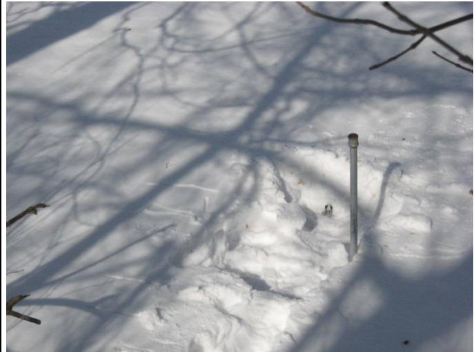
Photograph 6. ↑ Mini-piezometer and staff gauge installed at east end of pond, facing west.
