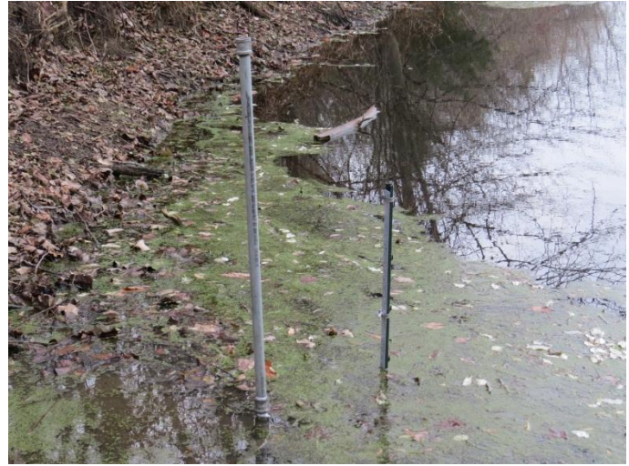
Photograph 6. ↑ Mini-piezometer and staff gauge installed at east end of pond, facing west.
