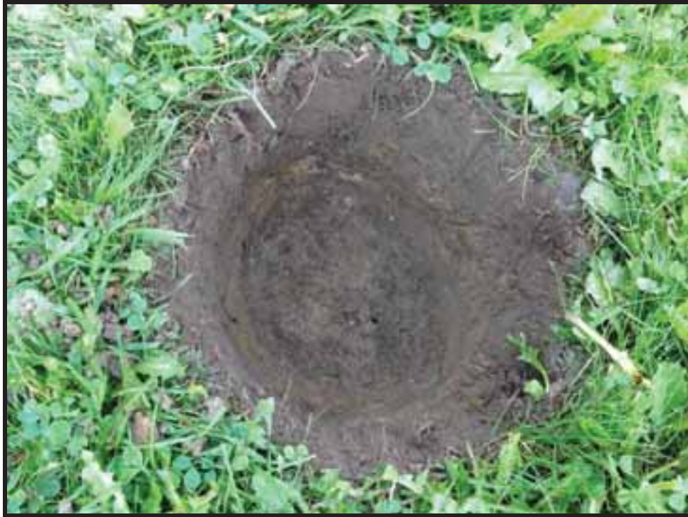
Image 47: View of Typical Test Pit Excavated into Subsoil at BLW1096 (Photo Taken on July 29, 2013)
