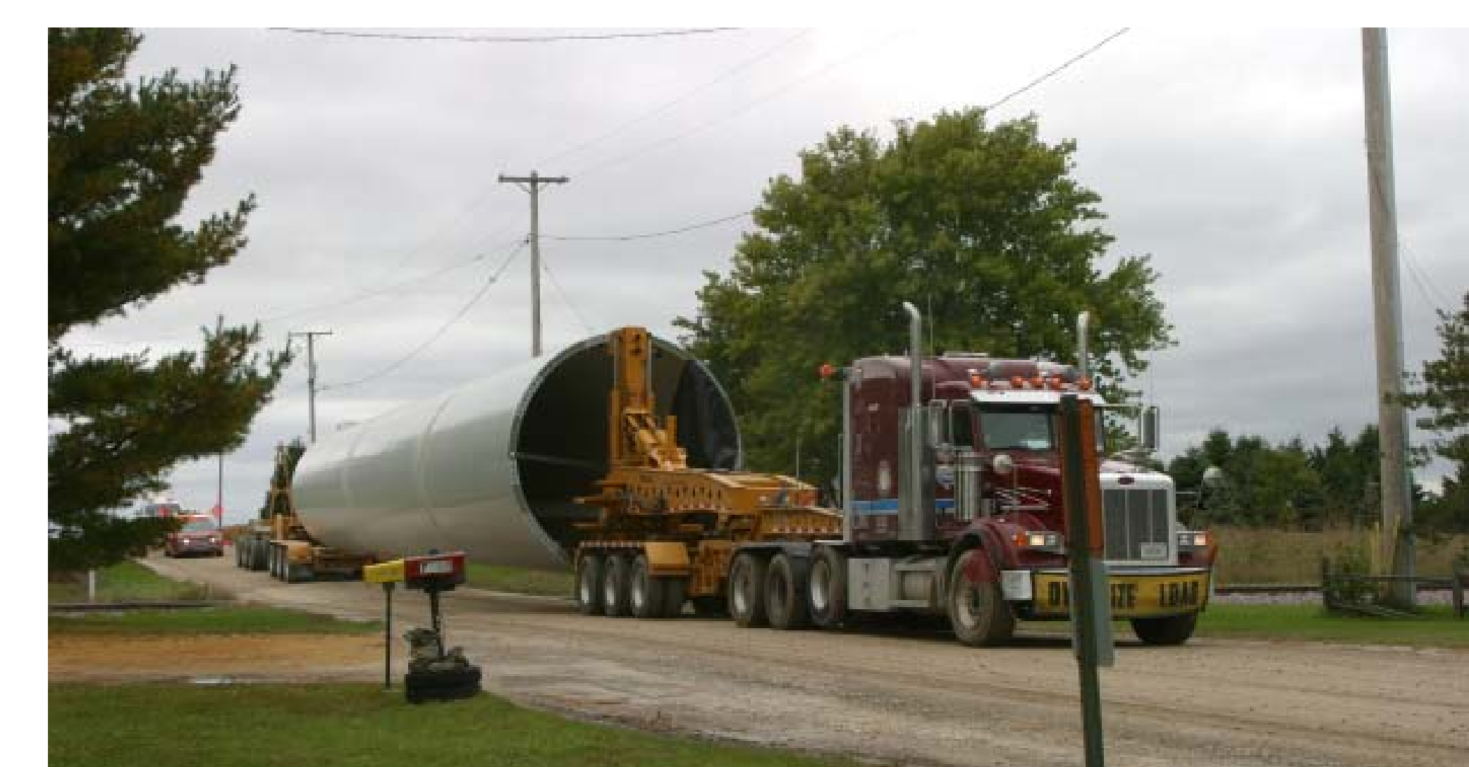
A tower section is transported to the site for assembly of a wind turbine.
