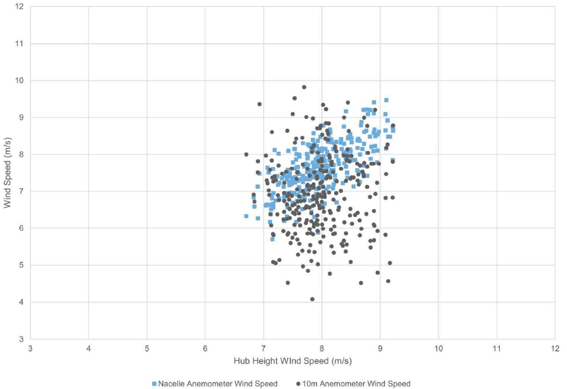
■ Nacelle Anemometer Wind Speed    ● 10m Anemometer Wind Speed
